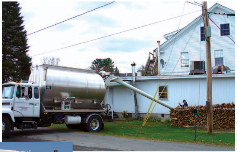
Nichols Hardware in Lyme, N.H., receives a delivery of wood pellets to be used as fuel for its 150,000-Btu-per-hour wood pellet boiler. The building has been heated entirely with biomass fuels for 30 years.
