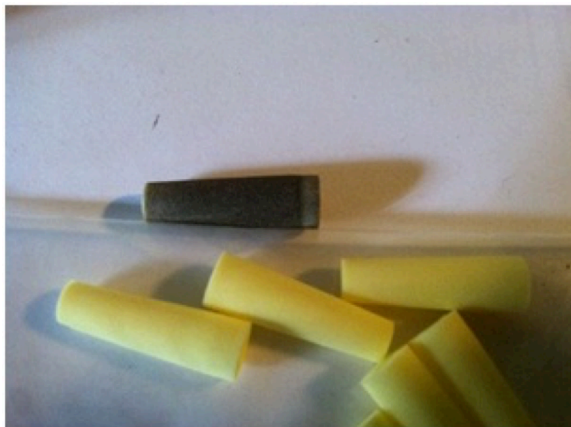
Figure 3. After several hours of use, the filter in the Testo gets dirty and needs to be switched out with a new one.
