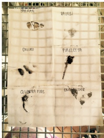
Figure 5. A sample of soot wiped off the glass of each stove shows a variety of consistencies and black and brown colors and build-up collected during glass cleaning.
