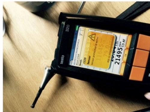
Figure 11. Testo 320 Gas Analyzer in “sensor protection” mode after attempting a high power test on the Harman.
