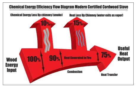
There are two aspects controlling the overall energy efficiency of a wood heater. First there is the combustion efficiency, i.e., how much of the wood fuel actually goes to the carbon dioxide and water end products of complete combustion rather than making smoke and creosote. Second is the heat transfer efficiency to the home of the energy that is produced by combustion.
