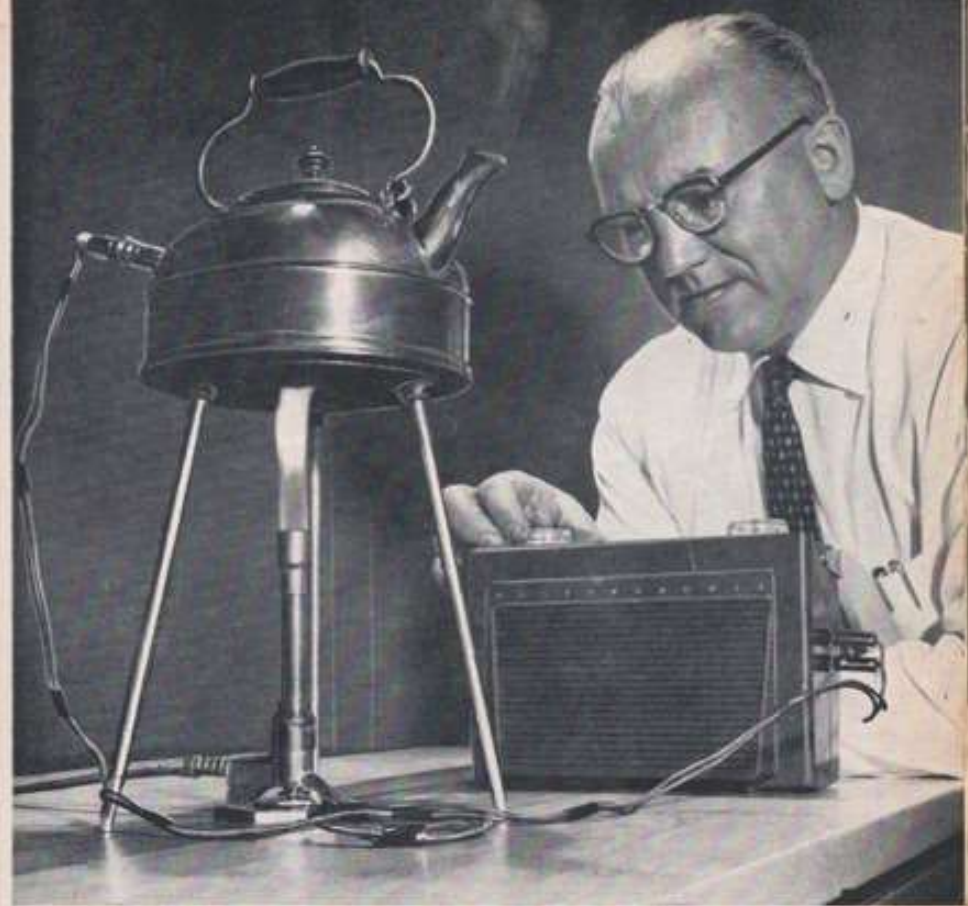
Using materials which change heat directly into electricity, this thermoelectric teakettle powers radio
